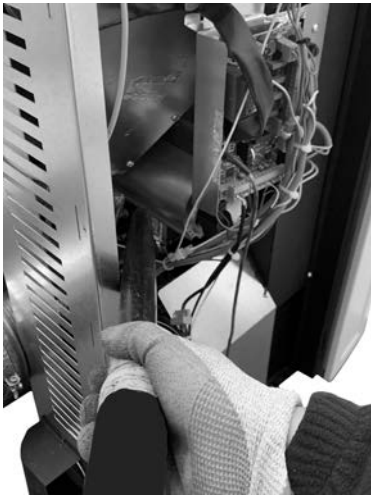
Fig. 108 - Reinigung Raumventilator (Atena 3 Plus 12/14 - Duke 12/14 At - Saba 12/14)
